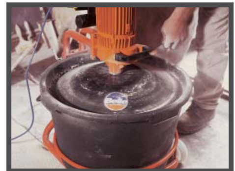
SPINNING DISC ENSURES SPLASH-FREE MIXING
